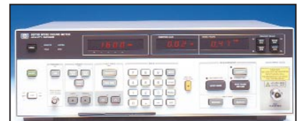
5. The HP 8970B NF meter has long been a precision tool for simultaneously characterizing the NF and gain of low-noise devices.
